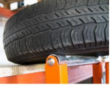
**OPTIONAL:** possibility of adding an arm with lifting ropes for stowing tyres flat. It helps to move the tyres from the tool to the shelf without lifting it. The operator doesn't make any effort and always keeps the correct position
