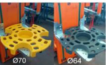
The forks pick up trolleys of different sizes
